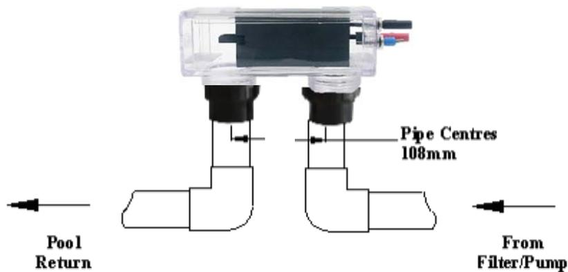
**WARNING:** It is essential that pipe work and equipment do not allow gases generated from the cell to collect and build up.
